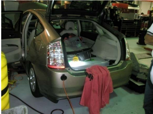
Plug-in Prius (5 kWh Hymotion pack)
